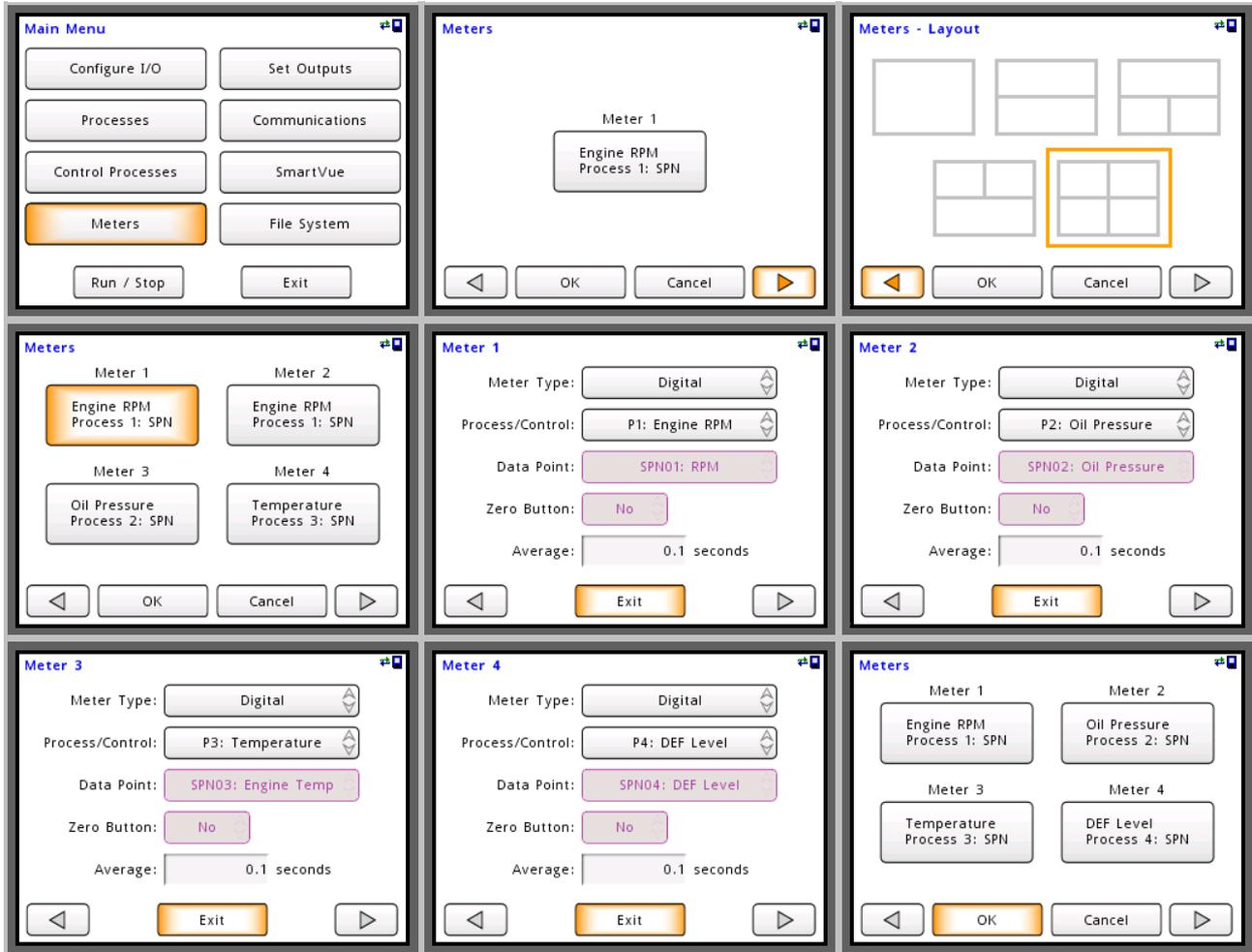
Now that all four meters are configured exit the “Main Menu” to view the meter screen. You should now see the RPM, Oil Pressure, Engine Temperature and DEF Level. If the communications is interrupted for more than the configured timeout of 10 seconds the meter screen will display “TIMEOUT” in red.
