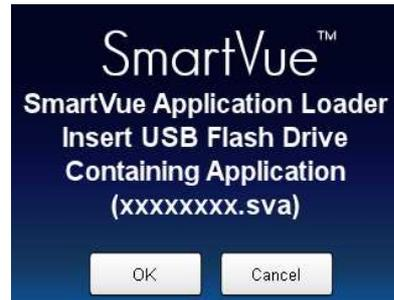
3. The Application Loader will detect the .sva file and display a message similar to the one shown below.
