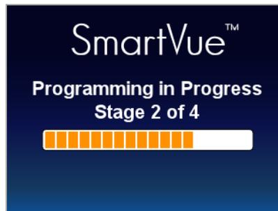
Once updating is completed, the SmartVue will prompt you to touch the screen so it can initiate a reset. During the reset you may see the message, “Uploading DSP firmware” at which time the digital signal processor firmware will also be updated.
